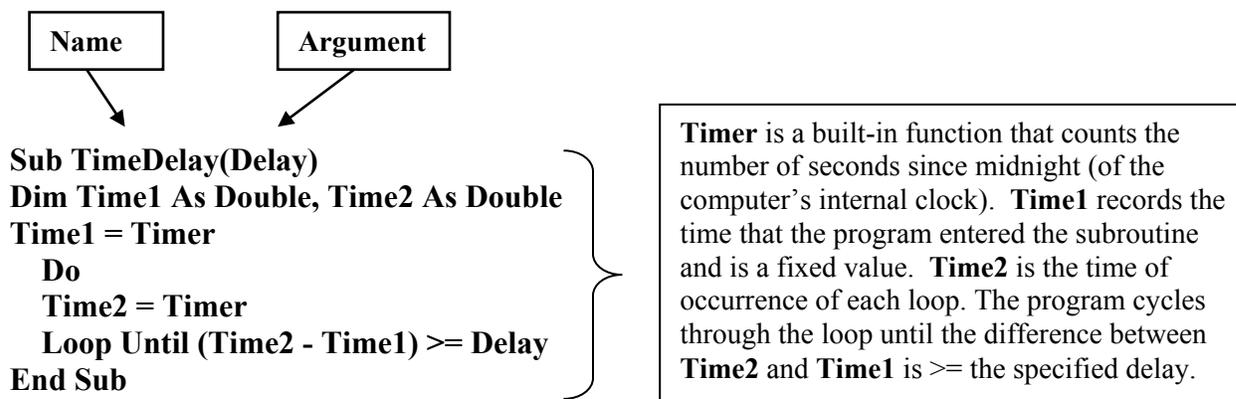
The subroutine is entered, or activated, by the statement **Call TimeDelay(Delay)** in the main program which transfers program execution to the subroutine. Once the **End Sub** line in the subroutine is encountered execution is returned to the main program.
